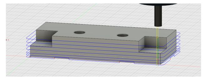
After all the toolpaths are set, I like to use the simulate button to watch the virtual CNC cutout.
