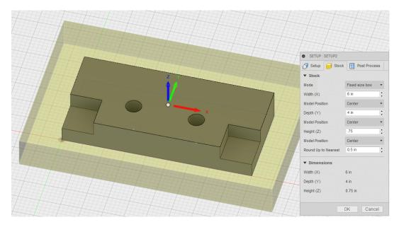
Next, I set the work coordinate system to match the KRMx02. To do this, I hit "Select Z axis/plane & X axis," and then clicking on a Z edge (any z edge will work)
