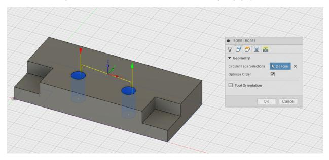
Next, I set the parameters for the holes (bit, feed rates, etc). Note: I don't have a SuperPID set up yet, so I'm just leaving Spindle Speed at the defaults. I set the cutting federate, lead-in federate, lead-out federate, ramp federate, and plunge feedrates. The others fields are automatically calculated
