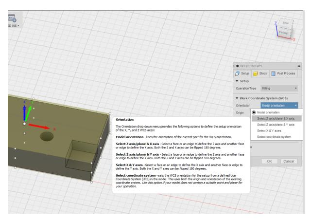
Next, I set the origin point by selecting "Stock box point" from the menu, then clicking on the lower left corner, on the top stock plane.
