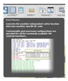
In the post-process window, I select "mach3mill.cps" from the post configuration menu, and select "No" on use G28. The rest is all default, unless you want to change where your output folder is.
