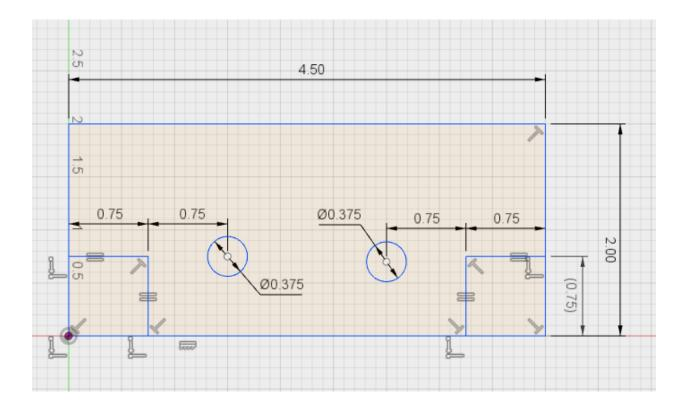
Here's where the workflow starts to deviate from VCarve... In the next step, I created a 3D model using the extrude command (again, great F360 videos showing how to do this), extruding the main body to 0.75" and the corner sections to 0.375. Looks pretty good!
